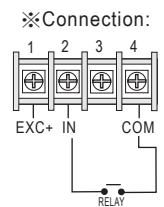
Relay Contact: NPN 0~100 Hz
