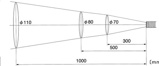
The optical resolution values stated in "Field of View" are at minimum 90% energy. The size of measuring object should be sufficiently larger than the field of view (spot size) shown in the above illustration.
