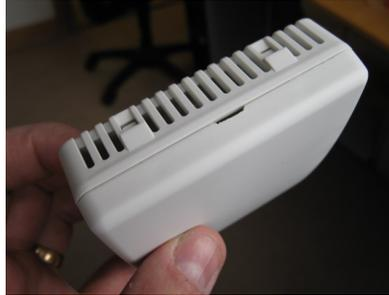
Figure 2. .By pressing a flat screw-driver into the opening slot, the two locking hook would be released.
