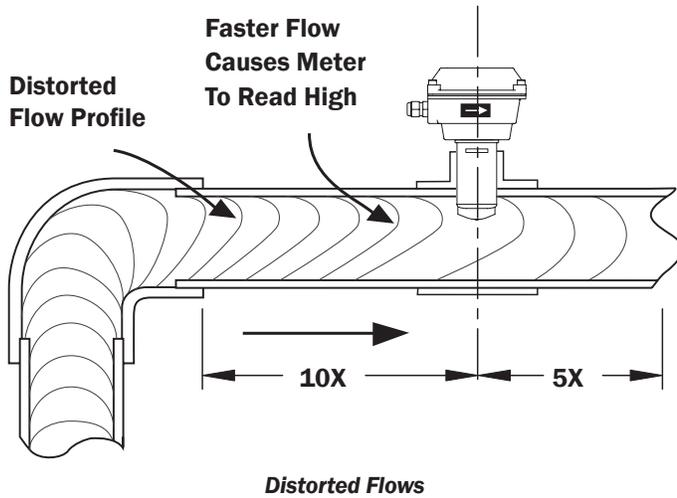
Although EX800-Series PVC meter tees are supplied with some straight pipe, additional straight pipe should be added to meet straight pipe recommendations. It is not advisable to connect a flow-disturbing device (e.g. valve or elbow) directly to the end of these fittings.
